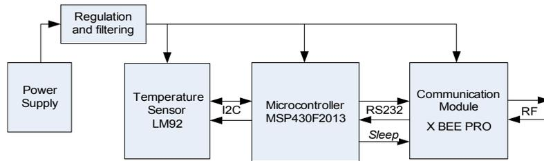
**Figure 3: Block diagram of the test micro-stations.**
